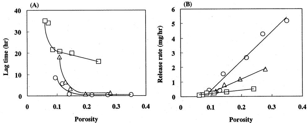
Fig. 2. Relationship between porosity and lag time (A) and porosity and release rate (B) in first fluid. Outer shell composition: (○) HPMCAS; (□) HPMCAS and CaSt; (△) HPMCAS and MgSt.
