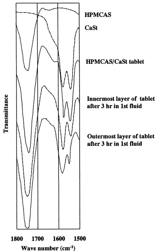
Fig. 6. IR spectra of tablets composed of HPMCAS and CaSt before and after immersion in first fluid.
