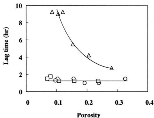
Fig. 8. Effect of porosity on lag time in second fluid. Outer shell composition: (○) HPMCAS; (□) HPMCAS and CaSt; (△) HPMCAS and MgSt.
