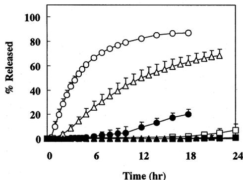
Fig. 1. Dissolution profiles of DIL from various press-coated tablets in first fluid. Compression force/outer shell composition: (○) 380 kg/cm<sup>2</sup>/HPMCAS; (●) 1530 kg/cm<sup>2</sup>/HPMCAS; (△) 380 kg/cm<sup>2</sup>/HPMCAS and CaSt; (▲) 1530 kg/cm<sup>2</sup>/HPMCAS and CaSt; (□) 380 kg/cm<sup>2</sup>/HPMCAS and MgSt; (■) 1530 kg/cm<sup>2</sup>/HPMCAS and MgSt. Each point represents the mean + S.D. (*n* = 3).
