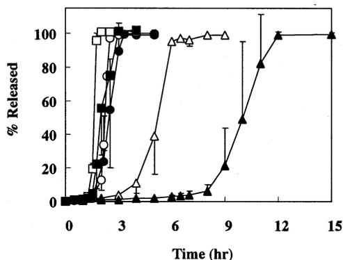
Fig. 7. Dissolution profiles of DIL from various press-coated tablets in second fluid. Compression force/outer shell composition: (○) 380 kg/cm<sup>2</sup> / HPMCAS; (●) 1530 kg/cm<sup>2</sup>/HPMCAS; (△) 380 kg/cm<sup>2</sup>/HPMCAS and CaSt; (▲) 1530 kg/cm<sup>2</sup>/HPMCAS and CaSt; (□) 380 kg/cm<sup>2</sup>/HPMCAS and MgSt; (■) 1530 kg/cm<sup>2</sup>/HPMCAS and MgSt. Each point represents the mean  $\pm$  S.D. ( $n = 3$ ).
