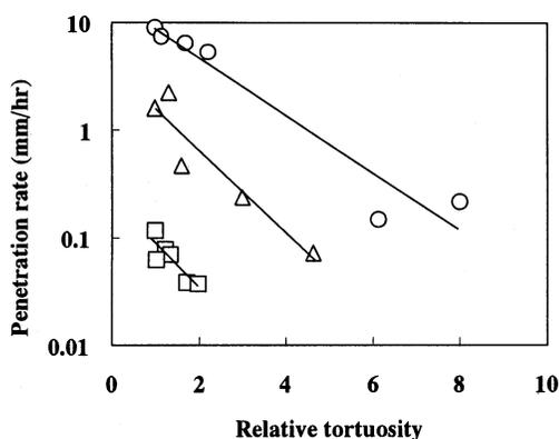
Fig. 3. Relationship between penetration rate and relative tortuosity in first fluid. Outer shell composition of press-coated tablet: (○) HPMCAS; (□) HPMCAS and CaSt; (△) HPMCAS and MgSt.
