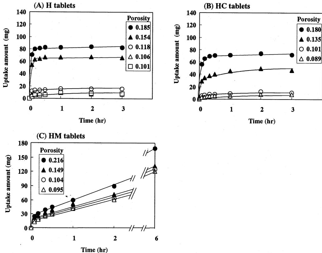
Fig. 4. Uptake amount of first fluid in tablets with various outer shell compositions.
