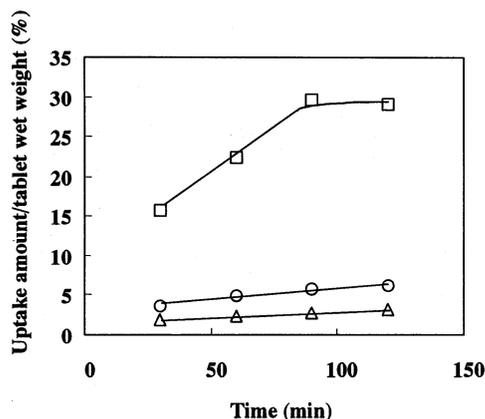
Fig. 9. Ratio of uptake amount of second fluid to tablet wet weight. Tablet composition: (○) HPMCAS; (□) HPMCAS and CaSt; (△) HPMCAS and MgSt.
